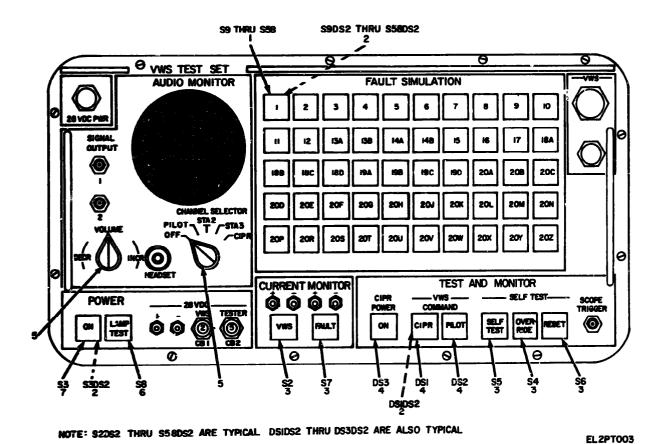
Figure 1. Reproducer-Converter Test Set AN/ASM-365.
